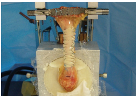
Figure 4 Simulated repair augmented with the DermaSpan ACD. Nine Lateral Trap Sutures were applied with continuous evenly spaced suturing per each medial and lateral side of the graft and were inserted into the graft approximately 5 mm from the medial and lateral edges.
