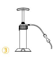
Connect vacuum tubing set. When vacuum is activated, vacuum indicator will collapse.
