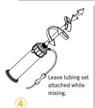
Mix cement by plunging handle up and down with rotating action. Mix cement thoroughly until the liquid and powder has formed a fluid mixture depending on the type of cement being mixed (minimum 30 seconds).
