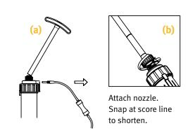
When mixing is complete, fully extend the mixing shaft. Snap off shaft. Remove vacuum tubing set. Attach nozzle. Snap at score line to shorten.
