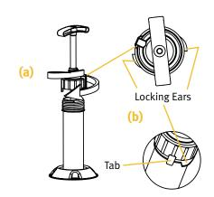
Thread cap assembly to mixing cartridge until tight. ENSURE THE CAP IS TIGHT AND TAB ROTATES PAST BOTH LOCKING EARS ON THE CARTRIDGE.
